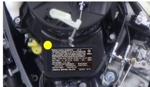
**NOTE:** Modified units still in their crate can be identified by blue seal marks on the labels as shown below:
