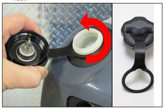
Install the new fuel cap by first screwing the plastic retainer (clockwise) onto the threads until it stops at the bottom of the threaded area. Install and tighten the fuel cap securely.
